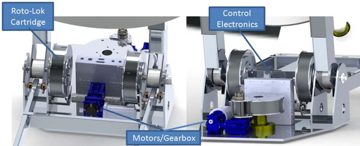
**Figure 3. Pedestal Concept, Key Components, and Modularity**
